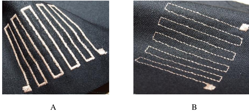
Fig. 2: Embroidered passive components, A) conductive pattern filled with many conductive threads, B) conductive pattern created with only one conductive thread.
