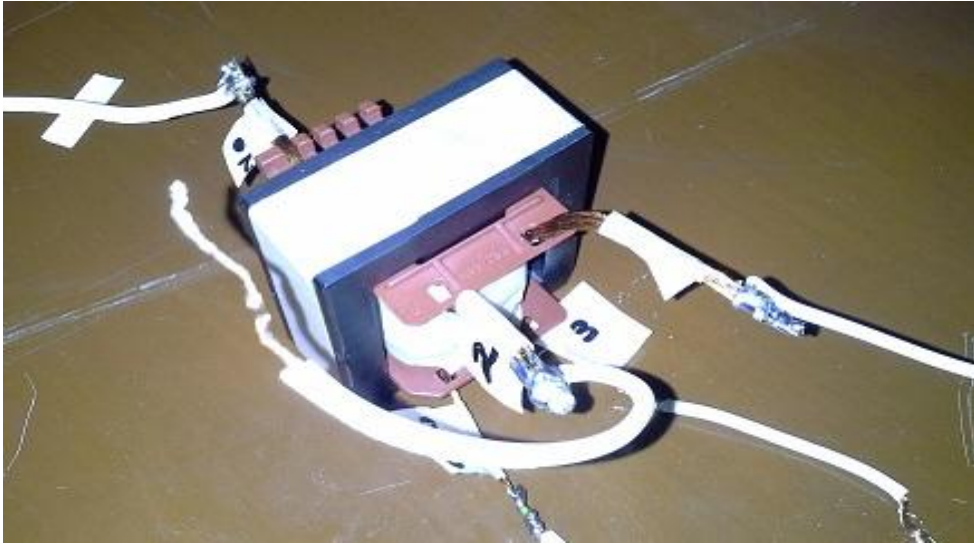
Figure 6: Undertest flyback transformer.
