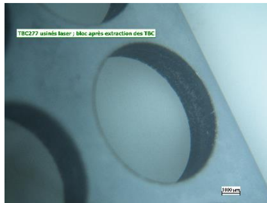
Laminated green block after laser machining, MLCC's removed
