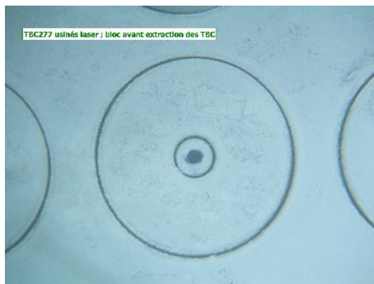
Laminated green block after laser machining, MLCC's still in place
