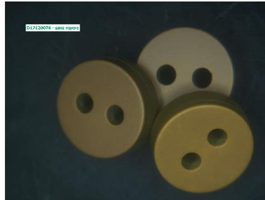
Laser machined circular MLCC's, fired, grinded
