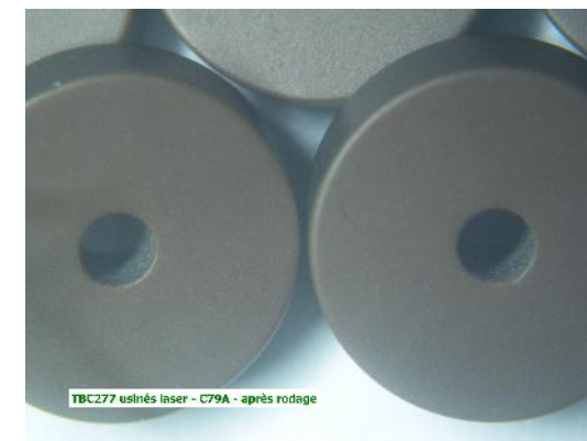
Laser machined circular MLCC's, fired, grinded
