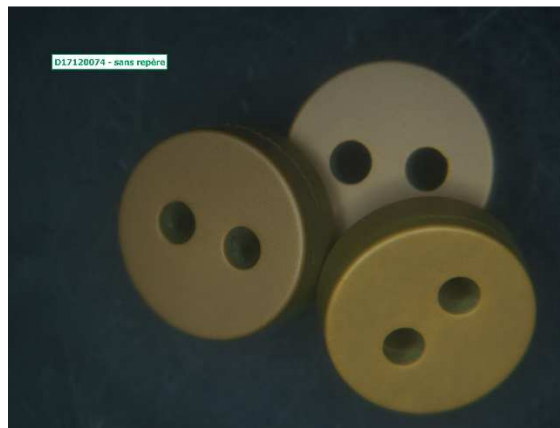
Fig.10 : 2-capacitances TBC after burn-out, sintering and corner-rounding
