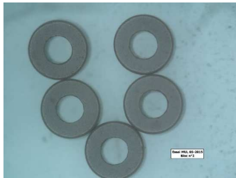
Fig. 1 : Circular miniaturized single capacitance model
