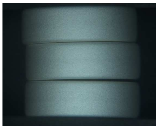
Fig.11 : 2-capacitances TBC after roll end termination
