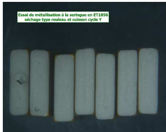
Fig.12 : end termination manual syringe deposit on 2220 parts
