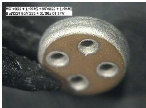
Fig.2 : Circular miniaturized multicapacitance model
