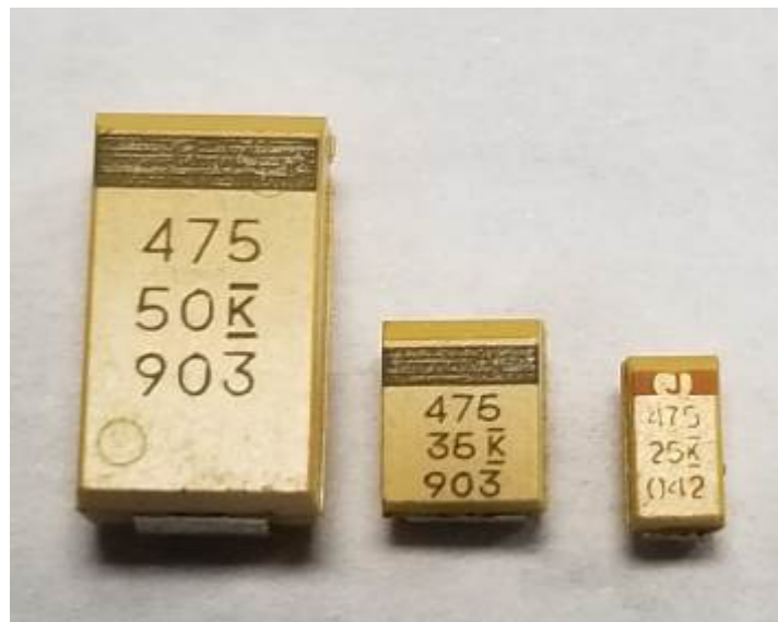
Fig. 6. Surface mount Solid Electrolytic Ta capacitors D-case 4.7 uF -50 V, B-case 4.7 uF – 35 V and A-case 4.7 uF – 25 V
