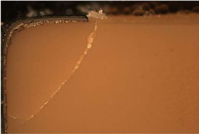
Figure 14. Optical Image showing flex cracking in a cross sectioned MLCC.
