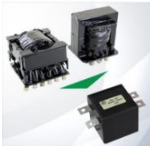
Figure 6 : Shapes of 2 discrete magnetic components (up) compared to final IMC (down)
