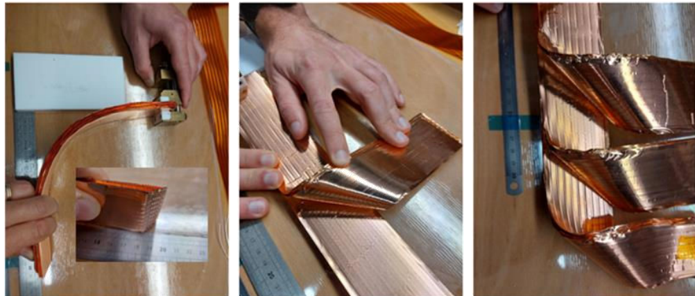
Fig. 8. Mock-up derisk on internal inter-tank harness.
