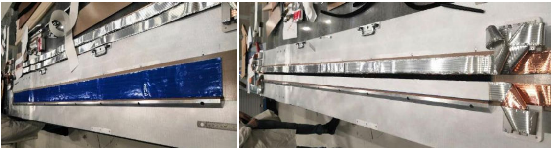
Fig. 19. Lay up of the a glue film (left), and the Flexible Conductor Cable underneath.
