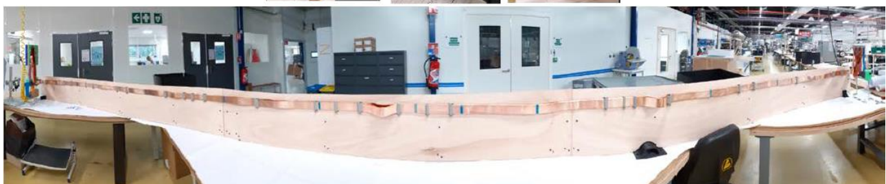
Fig. 16. Harness integration test (above) and final result on a 9 m long internal inter-tank mockup (below).
