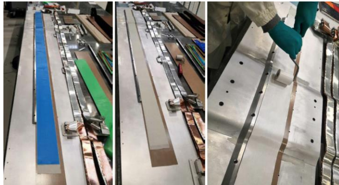
Fig. 18. Lay up of the first composite layers (in groups of 7) and application of the roll.
