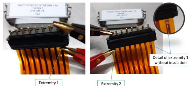
Fig. 22. Example of electrical resistance testing between contact and FFC.
