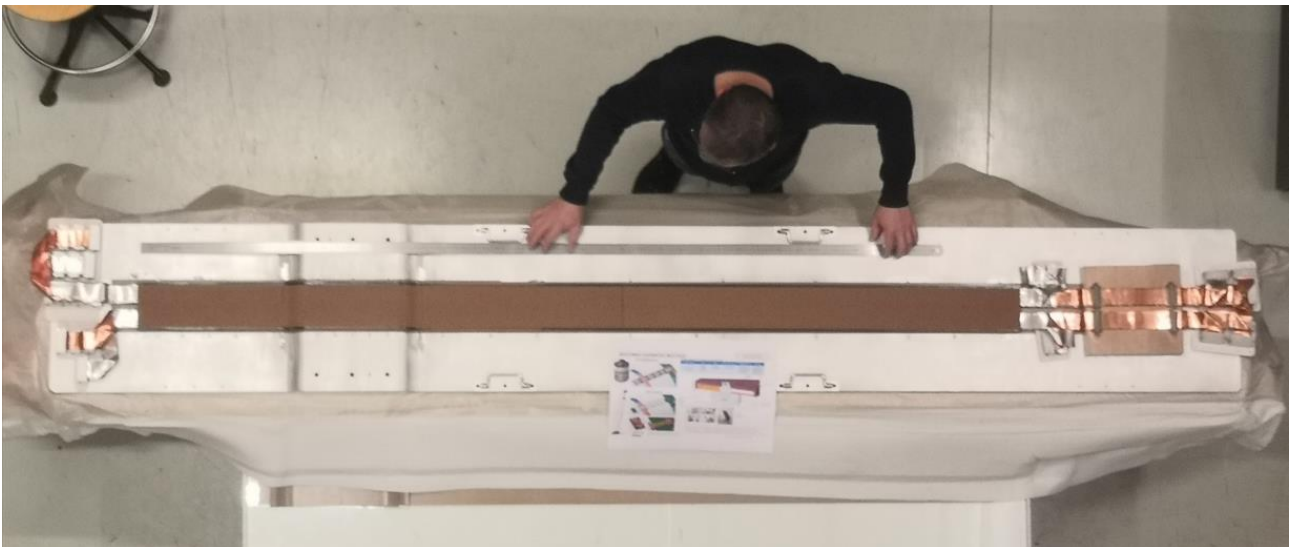
Fig. 21. The final mock-up as a single electro-mechanical part (Electro-Structural Composite).
