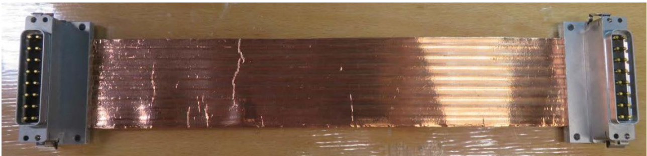
Fig. 14. Mating of the FCC with the connectors.
