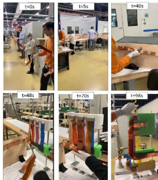
Fig. 15. Final Harness checking.
