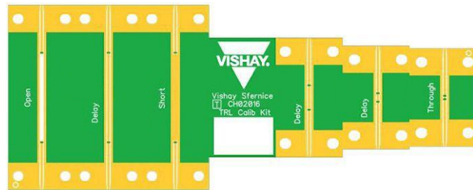
Fig. 6 - Thru reflect line calibration board
