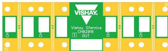
Fig. 7 - DUT characterization board
