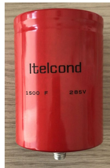
Figure 9. Final SC-GN3 "zero prototype" of wound supercapacitor with 1500F / 2.85V active element inside
