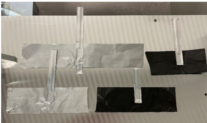
Figure 8. Sample electrode termination tab connection
