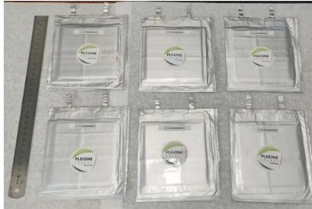
Fig. 1. Assembled Supercapacitor cells
