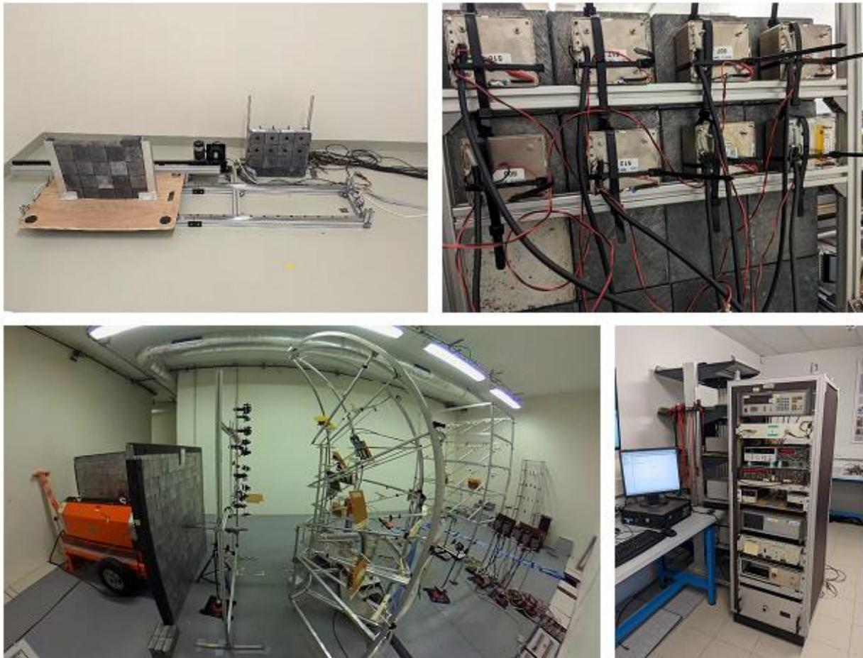
**Fig. 9: Lead shield with holes with the movable wall (top left), oscillators on the lead wall from behind (top right), gamma source (bottom left), measurement system (bottom right)**
