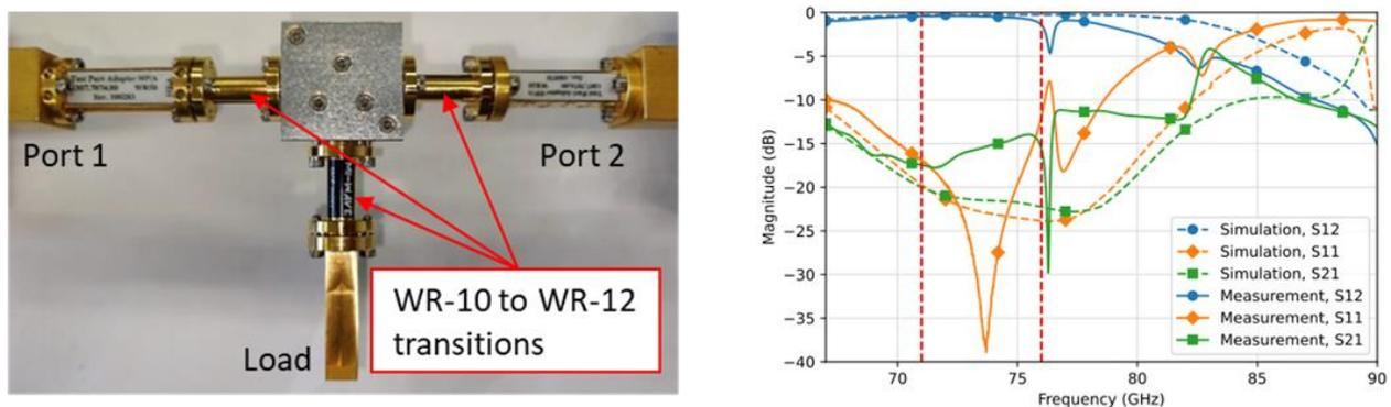
Fig. 3. Measurement setup (on the left) and comparison of simulated and measured S-parameters (on the right).
