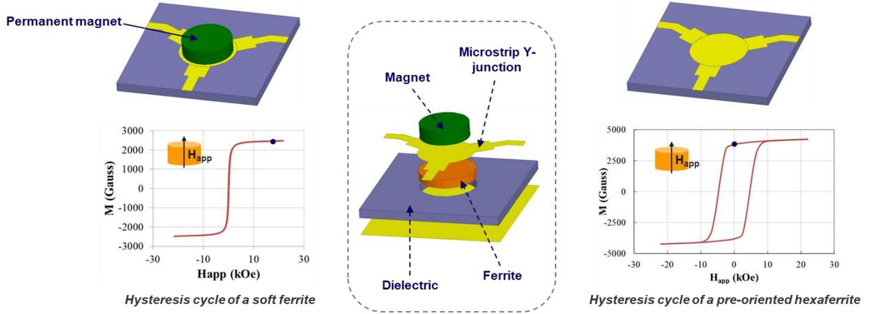
Fig. 1. Illustration of the structure of a standard circulator using a soft ferrite (on the left) and of a self-biased circulator using a pre-oriented hexaferrite (on the right).
