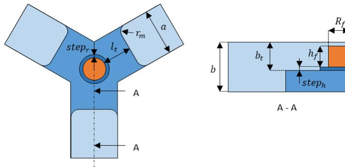
Fig. 2. Drawings of the rectangular waveguide Y-junction circulator.
