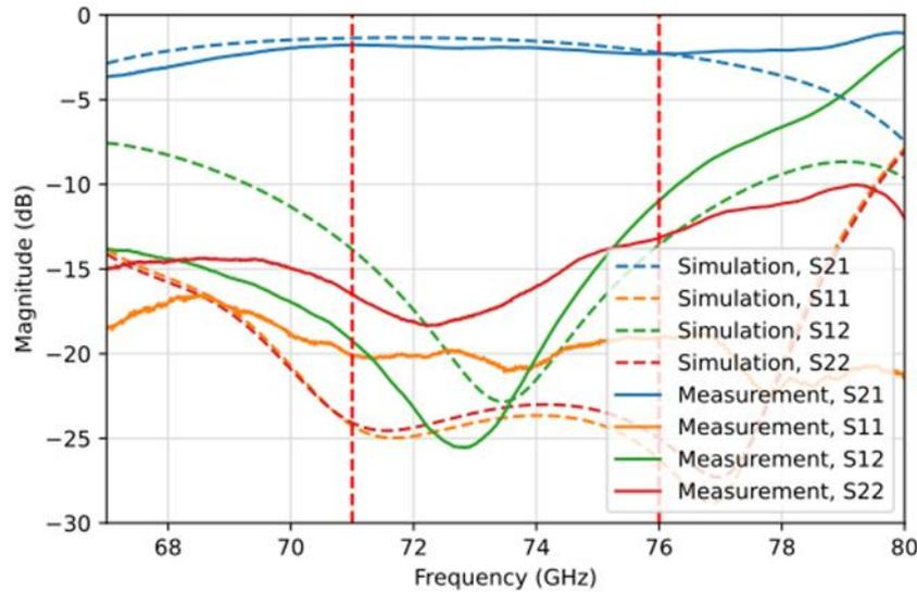
Fig. 5. Comparison between simulated (short dash) and measured (full line) S-parameters of the W-band planar isolator.
