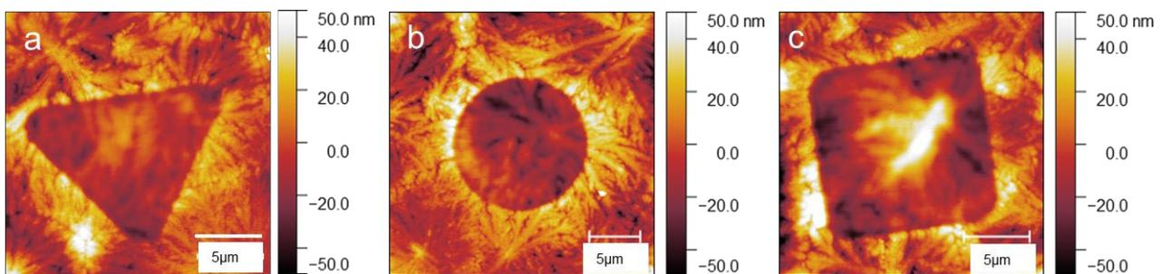
Figure 2. Different shaped a) Triangular, b) Round, and c) Square-shaped AFM images of the spin-coated PP film after He<sup>+</sup>-FIB irradiation with the dose  $5.4 \times 10^{-5} \text{ nC}/\mu\text{m}^2$
