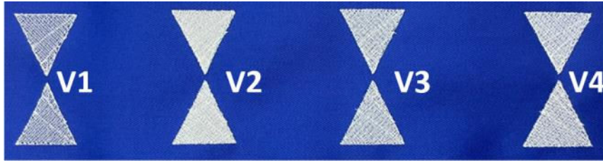
Fig. 9. Bow-tie antennas with different embroidering densities.
