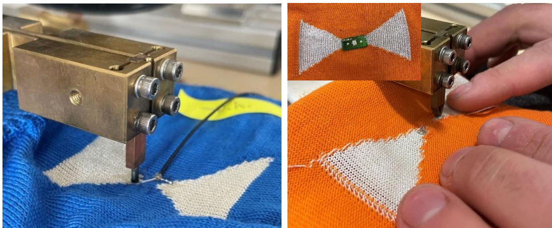
Fig. 7. (A) Hot bar spot welding of SMA pigtail and (B) PCB hot bar spot welding.
