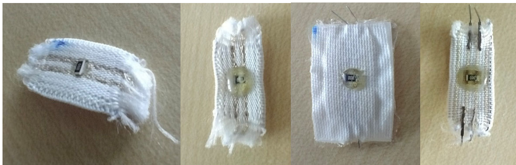
Figure 8 Samples after 30 washing (from left to right without protection, basic, additional protection, insulation)
