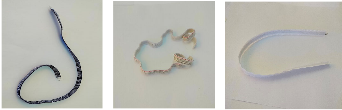
Figure 5 Samples of ribbons from left insulated, uninsulated, additional protection
