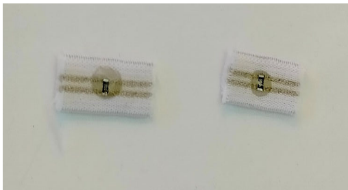
Figure 2 Samples with basic protection
