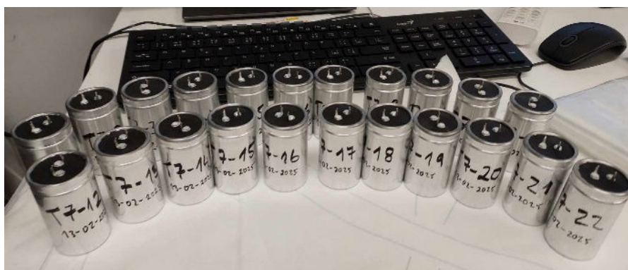
Figure 3: Finished prototypes with 70 cm long electrodes before submission to a test house for certification.
