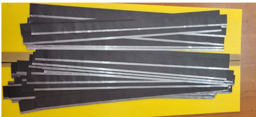
Figure 2: Electrodes fabricated and prepared for integration into wound cell prototype assembly.
