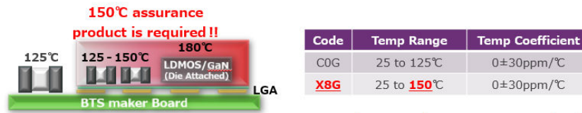
Fig.7 150°C rated products with voltage derating capabilities enables reliable operation in elevated temperature environments while maintaining capacitance stability
