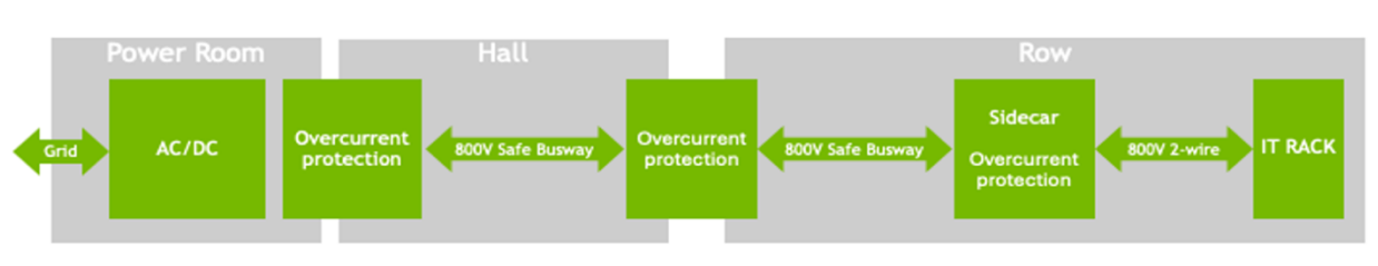
Figure 4. NVIDIA 800 VDC architecture minimizes energy conversions; source: NVIDIA [21]
