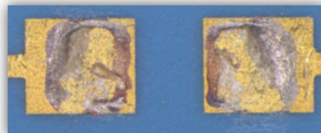
Figure 9 Views after Die Shear test. Silver Epoxy is observed
