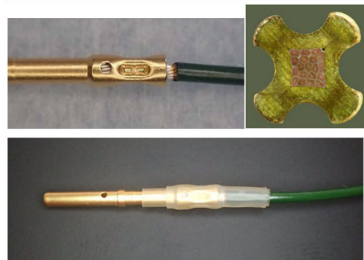
Figure 5-2: Example of a typical connector barrel and single wire crimping
